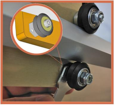
Turn the two eccentric screws to tighten the pulleys to the rail. Be careful not to over-tighten, the rail must be able to slide freely.
