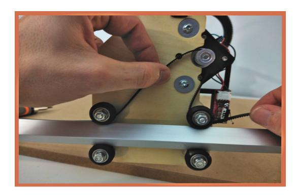
Place the belt around the stepper motor pulley.
