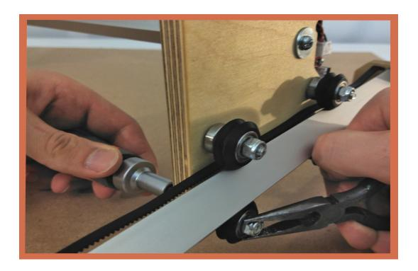
Lock the position by tightening the center screw.
