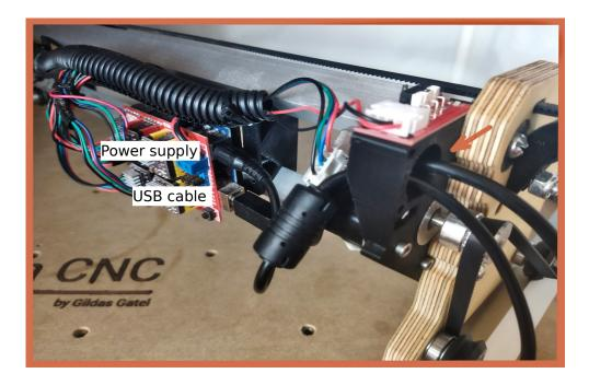
Connect the power supply and the usb cable to the motherboard passing through the ring.
