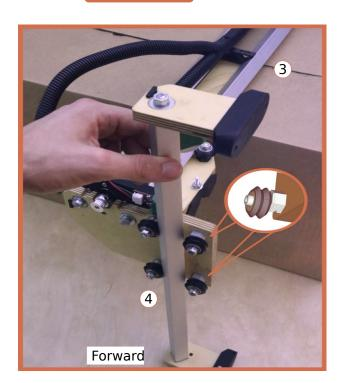
Install the rails on the gantry with the eccentric screw marker facing down. Pay attention to the direction of the rail.
